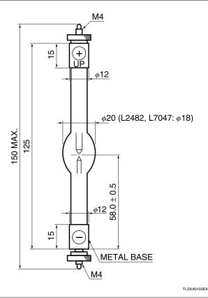
Super-Quiet Xenon Lamp: L2479, L2480 Super-Quiet Mercury-Xenon Lamp: L2483, L2917, L8288
